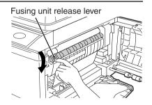
Gently remove the misfed paper from under the fusing unit as shown in the illustration. If the paper cannot be removed, proceed to "C: Misfeed in the transport area".
